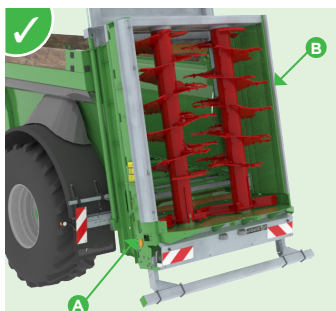
2 vertical beaters Ø 1,010 mm with continuous spiral on 219 mm tube: 423 rpm with a 1,000-rpm P.T.O. shaft drive.
