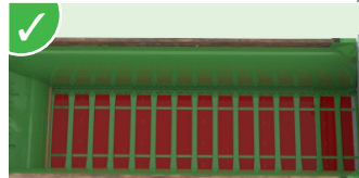
Floor in 4 mm high tensile steel with welded wear rails in 6 mm high tensile steel.
