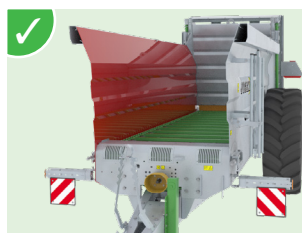
Narrow body made of 4 mm sheet metal (S420MC) with reinforcement folds over the entire length.
