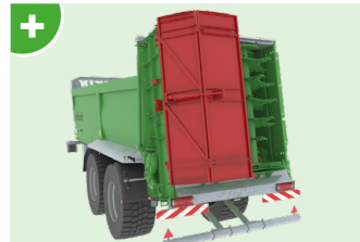
✓ Large hydraulic limitation board (right, left or both sides).
