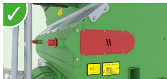
✓ Mechanical moving floor tensioner (using traction).
