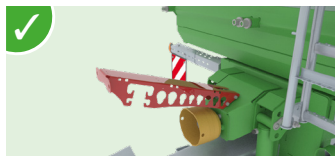
✓ Storage holder for hydraulic and electrical lines.
