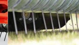
In extremely uneven conditions the optional centre gauge wheel prevents pick-up tines from digging into the soil. The robust steel roller only has ground contact when there are bumps underneath the centre of the pickup, lifting it up to avoid tine damage. The roll design guarantees that the pickup travels smoothly preventing it from bulldozing. The wear of the tines on uneven terrain is lower, resulting in higher forage quality and less contamination.
