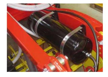
In order to brake the machine itself, the pneumatic brake can be mounted on the GP 600 M1 (Attention: 2-conductor pneumatic brake system must be available on the tractor!).
