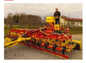
This additional equipment allows the user to drive the GP 600 M1 at 40 km/h (MOT-tested). Differences from regular version: Wider tyres, stronger brake, parking brake, light support with lateral delimitation lights, lateral yellow reflectors, 2 chocks, cover for lateral harrow sections.
