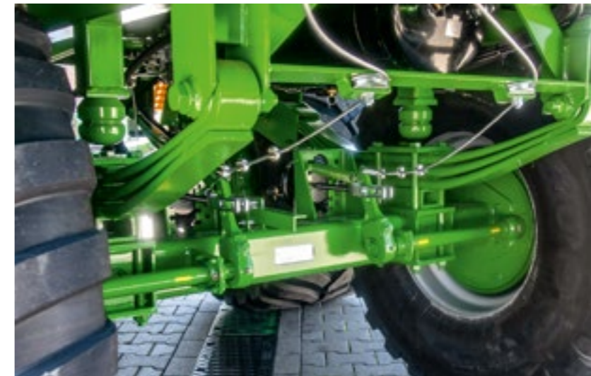
The drawbar and knife beam can be easily adjusted on the left side of the vehicle.
