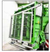
Protection grate for the beaters with hydraulic opening upwards (compulsory in some countries). On some models, the limitations boards can be combined with the rear grate.
