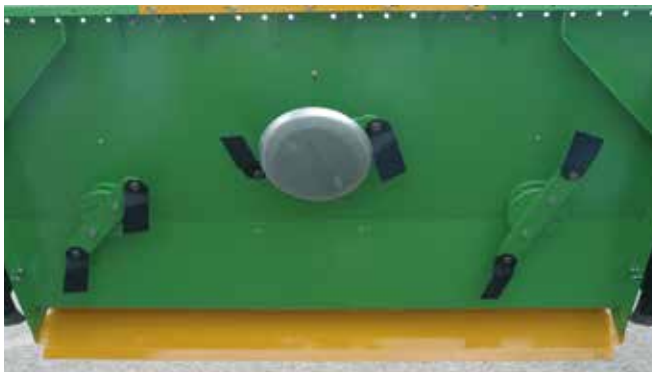
The TR pasture toppers are fitted with several small rotors (2, 3, 4 or 2 x 3). Each of them is fitted with two retractable blades of the D type which can turn on 360°.
