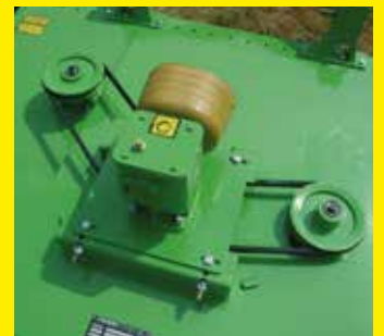
The different rotors are driven by 2 V-belts.
