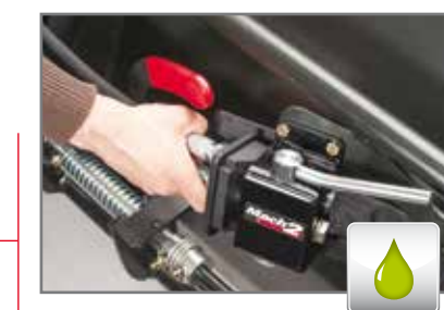
Instant connection of loader to implement hydraulic lines with the MACH 2 System®.
