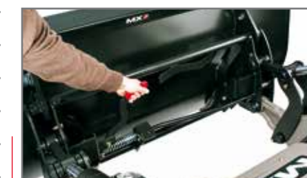
Automatic locking implement carrier: Well positioned release handle.
