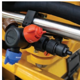
Triple nozzle with air shut off
