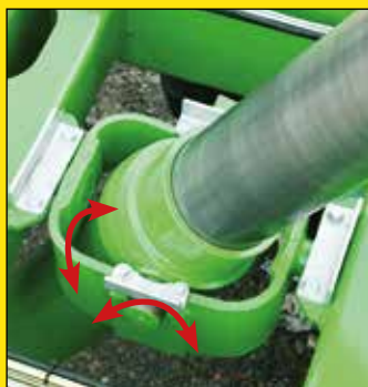
Double oscillating frame in which the ram is placed
