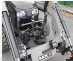
The chassis side brackets and hydraulic control valve are all shared between the MX loader and MX front linkage, making your tractor even more versatile.
